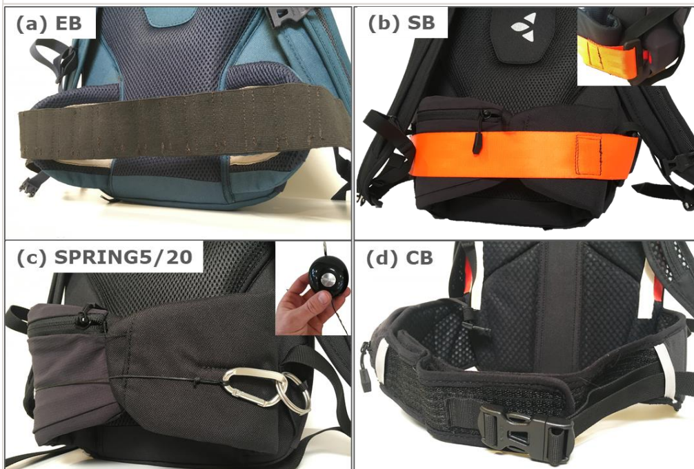
Fig. 1: Belt conditions: a) Elastic Band (EB), b) Seatbelt (SB), c) Spring balancer (SPRING5 & SPRING20), d) Conventional Belt (CB).
