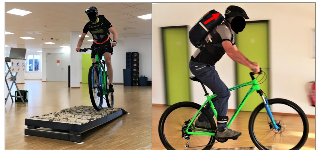
Fig. 2: a) Experimental set-up: Subject biking over the ramp. b) Visible backpack displacement indicated by white stripes
