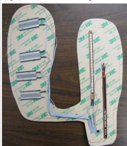
Fig. 2: Sensor layout for a miniature DAQ system: (left) force sensing resistors (FSRs) and (right) bend sensors on a ski glove insert
