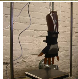
Fig. 5: Drop-test apparatus utilizing an instrumented, anatomically correct arm and force plate
